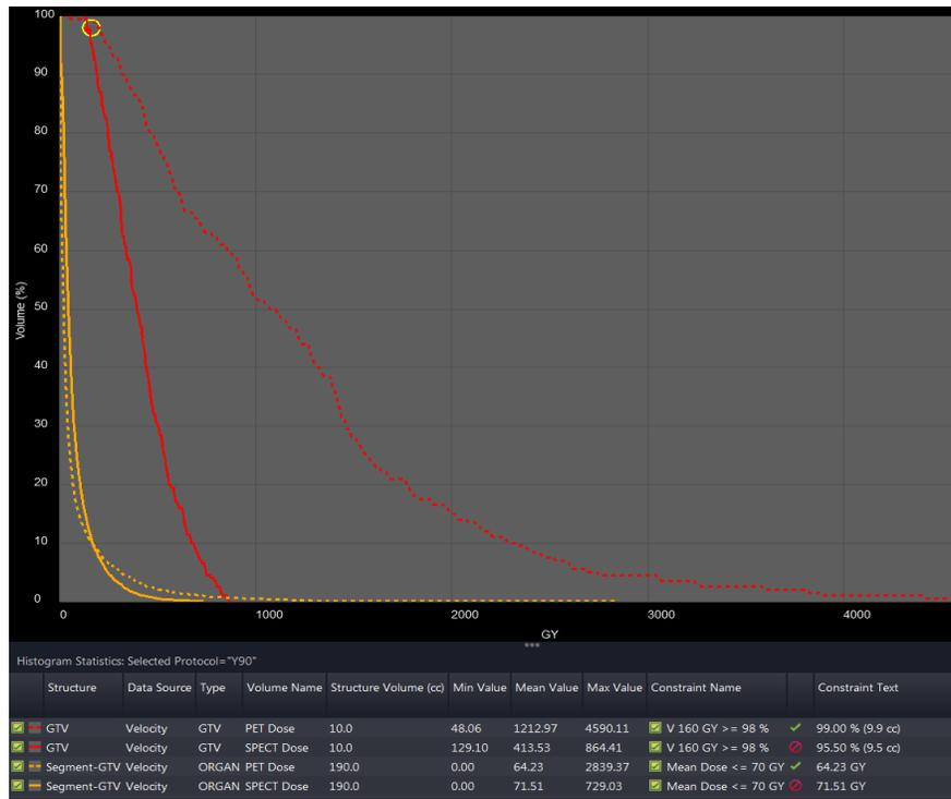
Figure 2: Dose-volume histograms for both SPECT (solid) and PET (dashed) dosimetry. The dosimetric goals were to cover at least 98% of the GTV with the prescription dose (V160Gy ≥ 98%) while keeping the mean dose to the rest of the segment (Segment – GTV) below 70 Gy. In this example, only the <sup>90</sup>Y PET dosimetry was able to satisfy the dosimetric goals. Also, the PET dosimetry method calculated much higher local doses within the GTV that are characteristic of brachytherapy.
