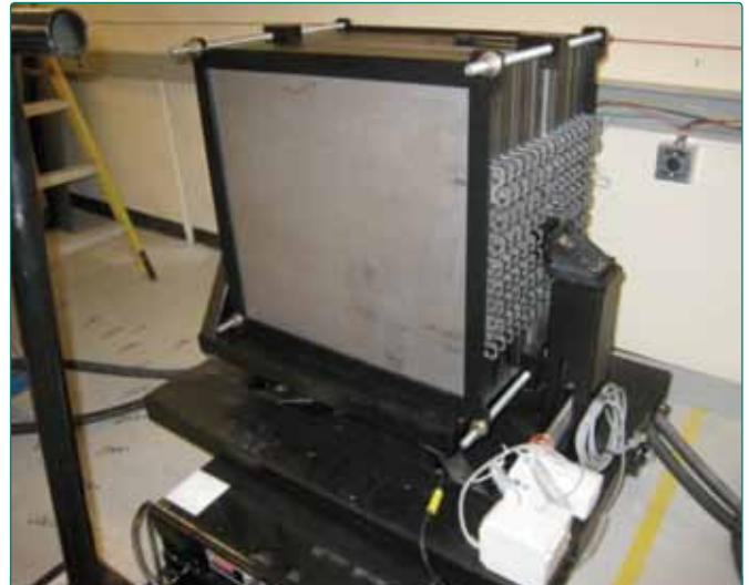
Figure 1. A test fixture with movable steel plates.
