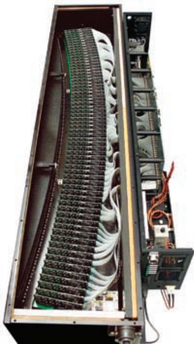
The digital detector array shown here is mechanically configured for use at a specific distance from the source, allowing each discrete detector board to maintain a consistent focal distance. Source: Varian
