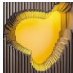
The Millennium multileaf collimator shapes radiation beams with 120 computer-controlled "leaves" or "fingers."
